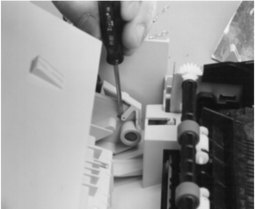
Figure 25. Printer door removal (3 of 3)
